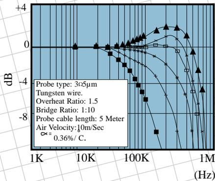
The typical frequency response graph was plotted according to data taken from AN-1003 Hot-Wire Anemometer with options 01 & 04. The amplitude is relative to the amplitude @ 1 KHz.
